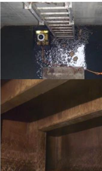
The Subsea Tech intervention team has inspected and measured the silt level of the 8 outflow reservoirs of the Cattenom Nuclear Power Plant, for SOCOTEC Nucléaire/EDF. A Cyclop type ROV fitted with video and acoustic camera has been used for this inspection. The HD PTZ video camera allowed inspecting the above water part and the BlueView acoustic camera to measure the silt level underwater.
